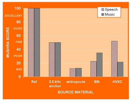
("w/dropouts") are "BAD" for both speech and music. With the graceful degradation scheme enabled, the audio quality is improved, with the speech material experiencing more improvement when the HVCX codec is used, and likewise for the music material with the SIN codec.
