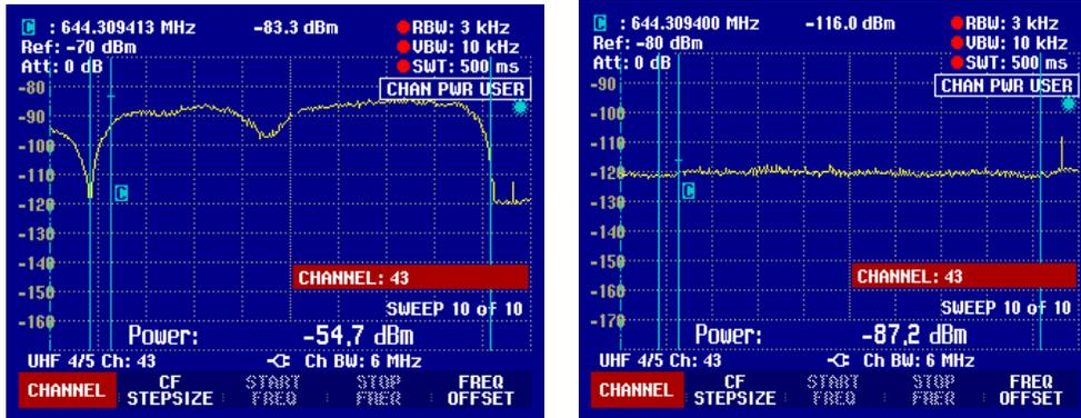
Both of these sets of measurements show locations and frequencies where spectrum sensing at levels below -114 dBm would result in harmful interference to nearby television reception.
