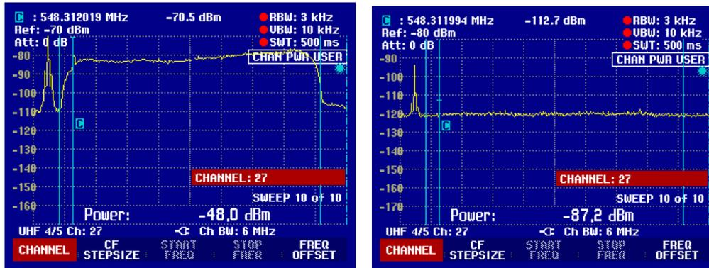
The above displays show the measured power of the pilot carrier on channel 27 at site 3 at both locations (Locations A and B). The pilot carrier power is displayed on the top center part of the spectrum analyzer display on the same line as the pilot carrier frequency.
