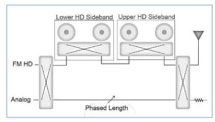
designated for either the analog or digital transmitter. The two input ports have a high degree of isolation between them, which helps keep unwanted emissions low. There are two output ports of the circuit. The first is the main output, which is where the highest percentage of the RF power flows. The second output is connected to a reject load. This load takes the remainder of the power that was not phased properly and turns it into heat, thus keeping reflections low and the circuit balanced.
