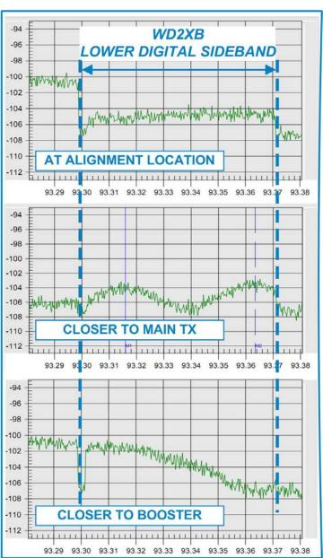
start to differ in both amplitude and delay, and the resulting spectrum exhibits the ripples and nulls that one observes when multipath fading is present. Even when this multipath distortion is present, the digital signal will still be receivable because of the OFDM system's resistance to multipath fading.
