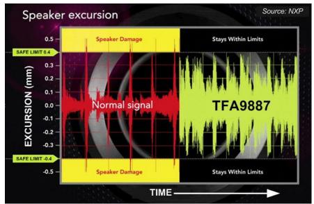
rule. Adaptive excursion control measures the actual excursion of the speaker membrane to ensure that it never exceeds its rated limit. Real-time temperature protection measures the voice-coil temperature directly to prevent thermal damage.
