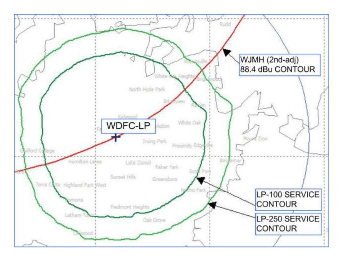
The figure above, taken from Appendix A of the Petition, shows an example of the impact of increasing the LPFM power from 100 to 250 watts for station WDFC-LP, Greensboro, NC. Also shown in the figure is the 88.4 dBu contour of 2nd-adjacent full-power station WJMH, Reidsville, NC (class C0, 102.1 MHz). Here are some of the details of the proposed rule changes (page numbers refer to the Petition document):
