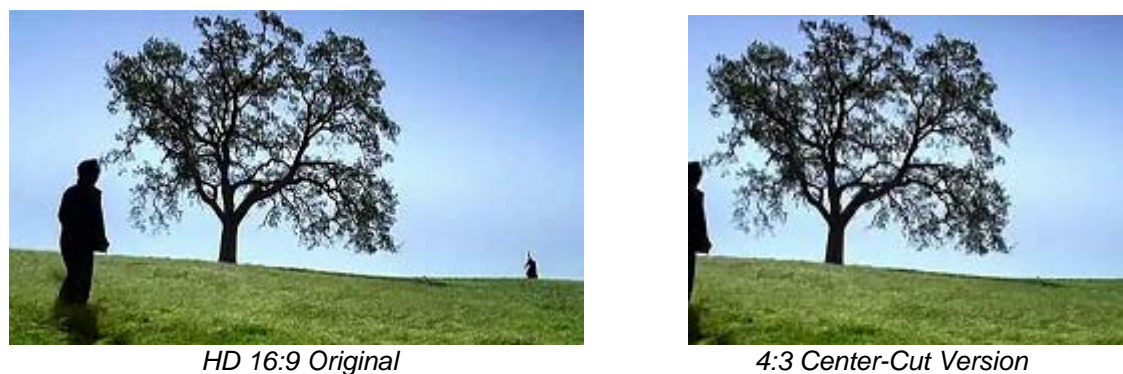
Figure 3: Example of Adversely Affected Center-Cut Down-conversion
